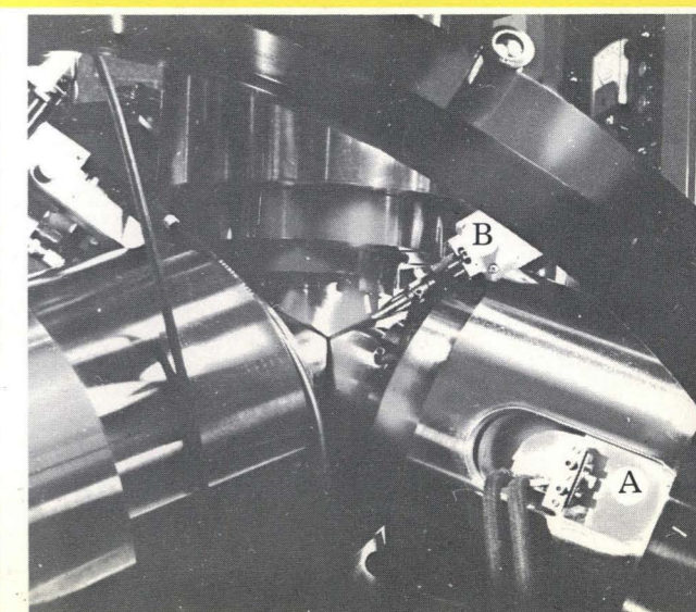
X-ray tube mountings from opposite side of photo No. 3. The upper (mount "B") has a collimator directed between the anvils to the sample. Lower (mount "A") shows x-ray tube mounted in the piston. Photo also shows optical piece for center alignment of anvils.
